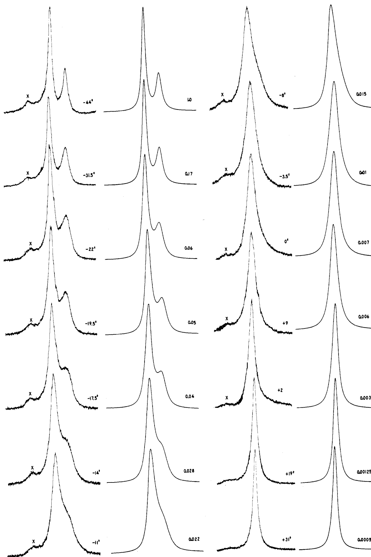
Figure 3. ^1\text{H} NMR spectra for [\text{Pd}_2(\text{CNCH}_3)_6](\text{PF}_6)_2 in acetone- d_6 as a function of temperature. Calculated spectra are shown to the right of each matching experimental spectrum. The lifetime ( \tau ) values for each calculated spectrum are given in seconds. The peaks marked "X" are due to an impurity in the sample.
